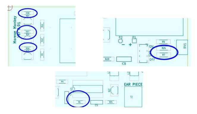
3. Next are 220 ohm resistors located at R2, R6, R3, R15, R14, R20, R21, R22, R23, R5.
