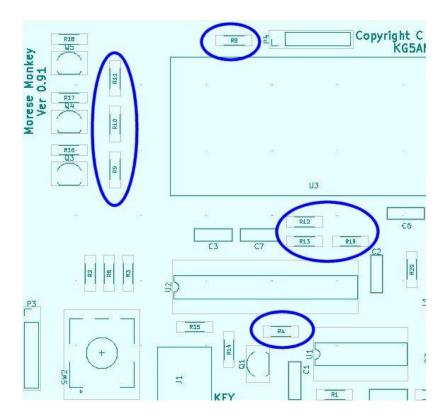
2. Next are 2.2K resistors located at R16, R17, R18, on the upper left, and R7, R24 on the lower right, R1 on bottom.
