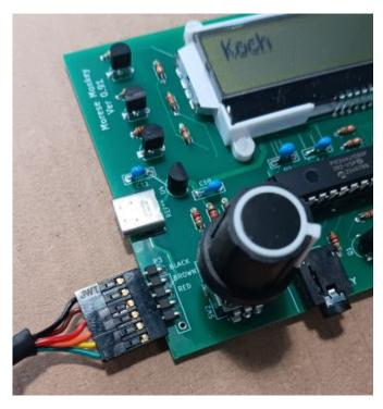
The cable is attached to a the header which is located by the selection knob. The black wire goes toward the back of the board, as shown.
