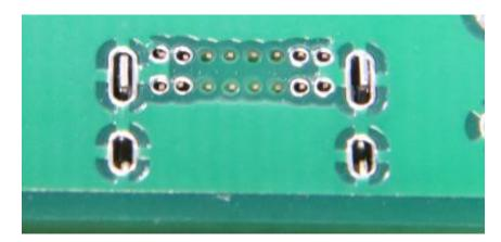
You can solder only the outer case, and the pins which are plated. The outer pins are physically connected to the case. Carefully heat them and flow a small amount of solder into the holes.
