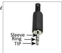
To connect a straight keyer, simply connect the keyer to either the tip or ring, and the sleeve as ground. The straight key contact is set the same as the lambic *long* (dah) contact, as described in the settings section below.
