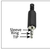
To connect an lambic keyer, the contacts are connected to the tip and the ring of the phone plug and the common ground is connected to the sleeve. The user can set which of the contacts (tip or ring) will produce the dah or long, and the other contact will produce the dit or short.
