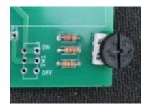
6. Turn the board over and carefully solder each lead, insuring not to short out to any adjacent traces on the circuit board.
