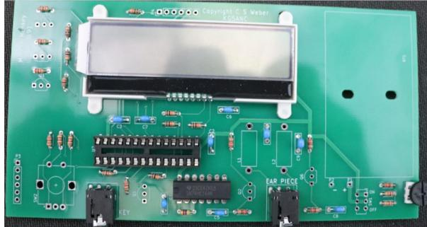
15. Next install the inductors, L1 and L2. Solder the inductors in place, and trim the leads.
