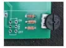
6. Turn the board over and carefully solder each lead, insuring not to short out to any adjacent traces on the circuit board.
