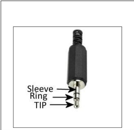
To connect an lambic keyer, the contacts are connected to the tip and the ring of the phone plug and the common ground is connected to the sleeve. The user can set which of the contacts (tip or ring) will produce the dah or long, and the other contact will produce the dit or short.
