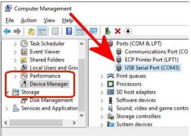
When the USB cable is attached to the PC, Windows will add a new COM port to the devices. You can locate the name of the COM port in the windows Device Manager, as shown here.
