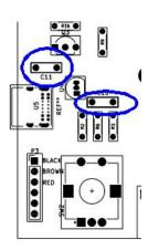
12. Last, install C1 located on the bottom next to U1 and solder it in place and trim the leads.
