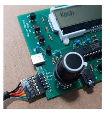
The cable is attached to a the header which is located by the selection knob. The black wire goes toward the back of the board, as shown.
