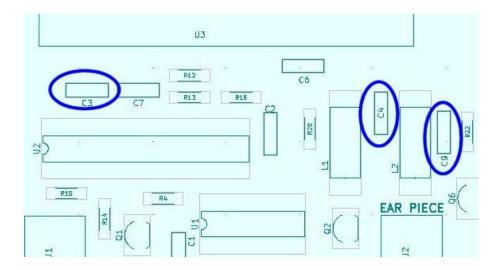
13. Last, install C1 located on the bottom next to U1 and solder it in place and trim the leads.
