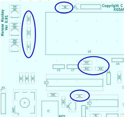
2. Next are 2.2K resistors located at R16, R17, R18, on the upper left, and R7, R24 on the lower right.
