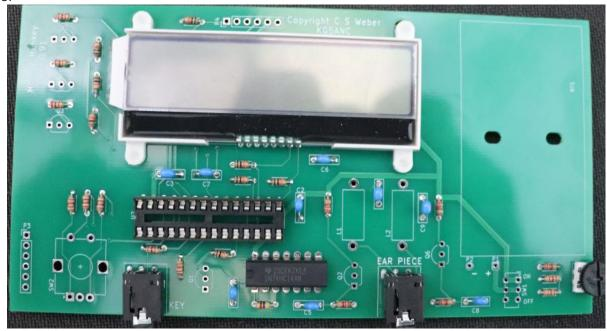
15. Next install the inductors, L1 and L2. Solder the inductors in place, and trim the leads.
