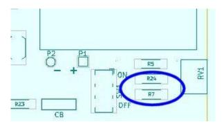
3. Next are 220 ohm resistors located at R2, R6, R3, R15, R14, R20, R21, R22, R23, R5.
