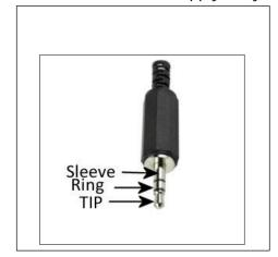
To connect an lambic keyer, the contacts are connected to the tip and the ring of the phone plug and the common ground is connected to the sleeve. The user can set which of the contacts (tip or ring) will produce the dah or long, and the other contact will produce the dit or short.
